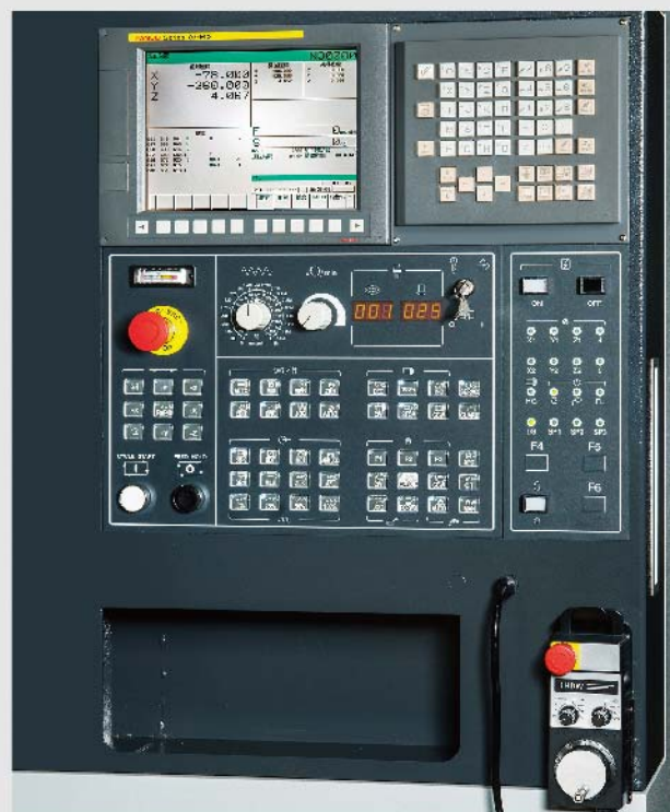
FANUC OI-MD 10.4" LCD + Manual guide I AICC II (200 blocks)
