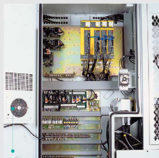
Heat exchanger is included as a standard accessory.
