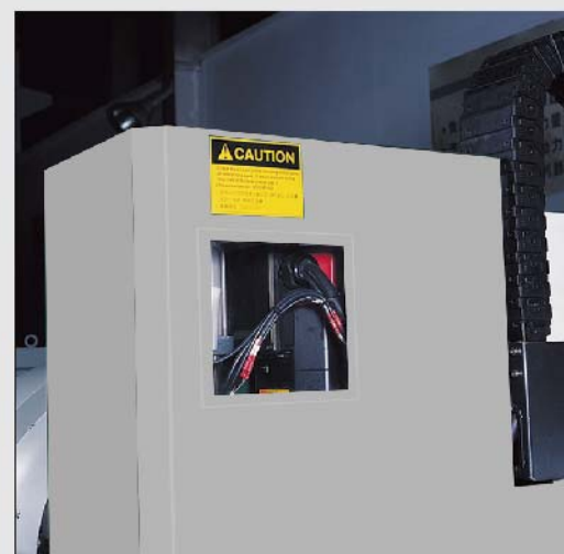
Transparent side window on headstock cover enables convenient inspection and maintenance.
