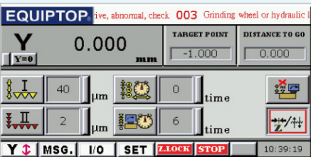
Grinding Condition Input
