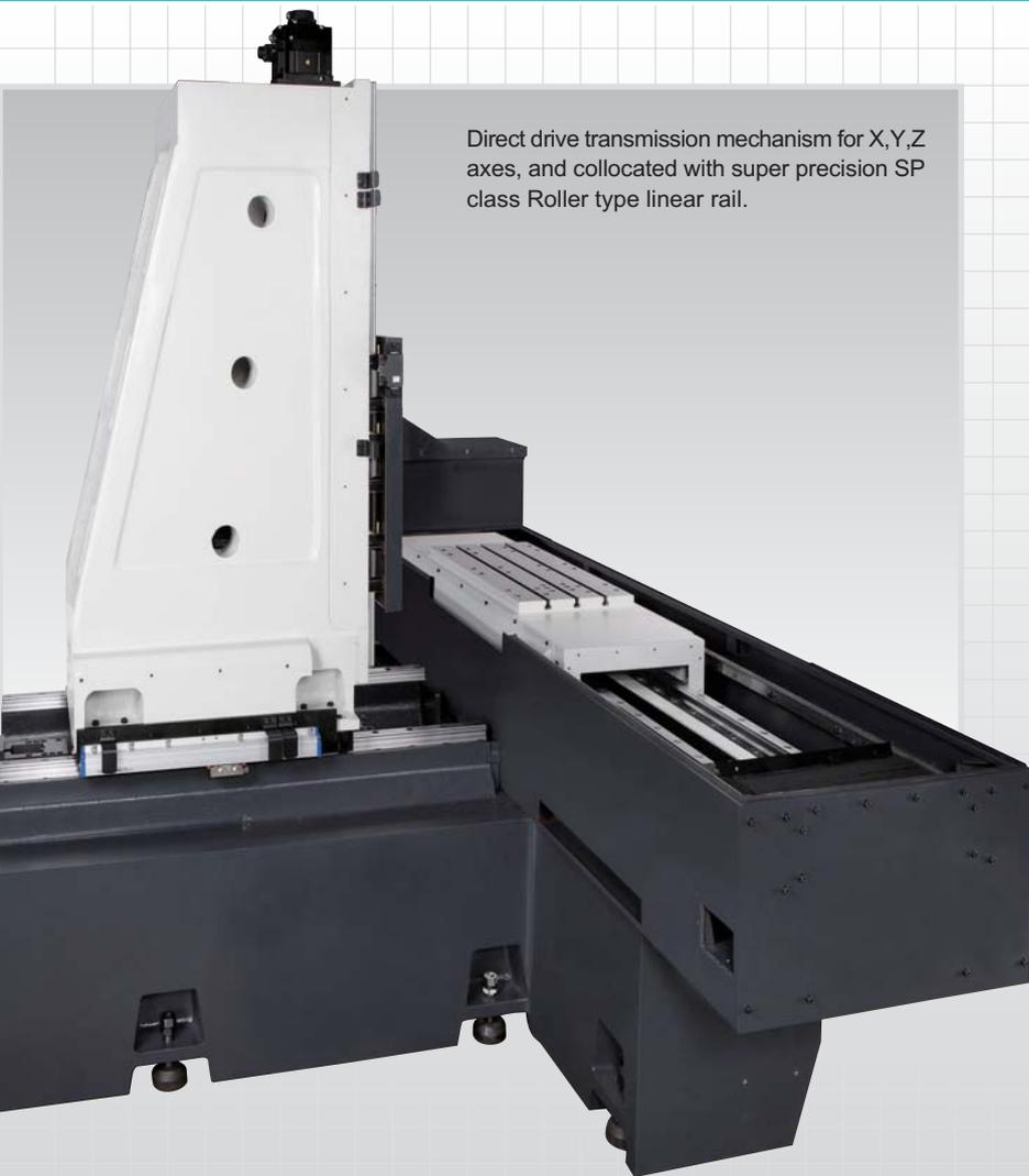
Direct drive transmission mechanism for X,Y,Z axes, and collocated with super precision SP class Roller type linear rail.
