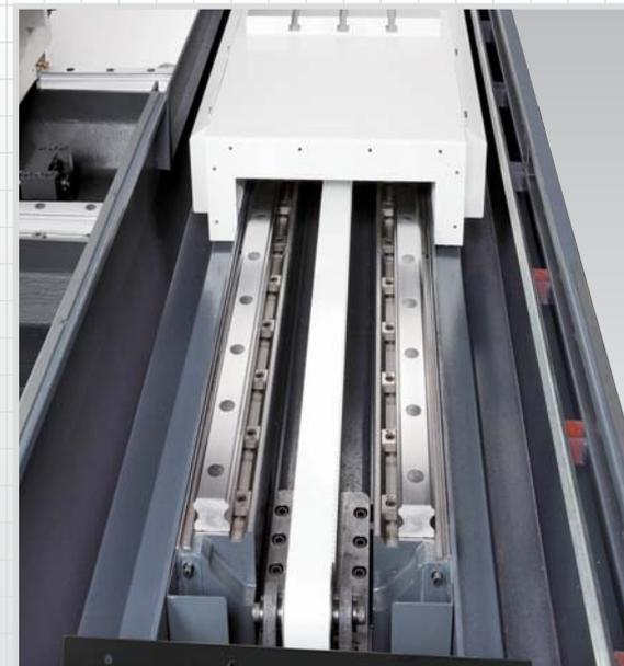
X axis direct drive transmission mechanism, collocated with super precision SP class Roller type linear rail. (Belt drive is available as option.)
