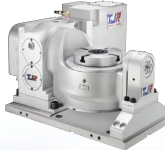
FAD-170F-RC210 (One D.D. Motor) Tilt axis : Driven by 80 rpm Roller Gear Cam Rotary axis : Driven by 300 rpm D.D. Motor
