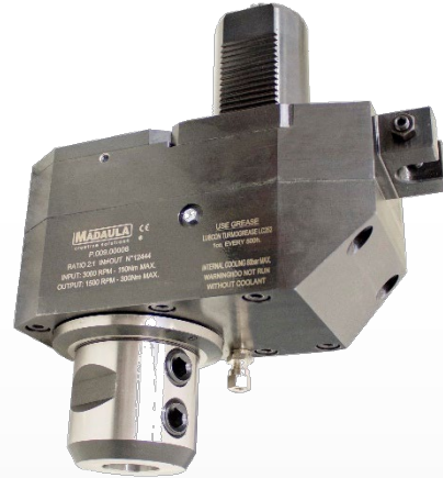
Axial Reducer IC for GORATU VDI-60 DIN-5482 / WELDON-32 Ratio 2:1 - IN≠OUT / 1.500 rpm Max.
