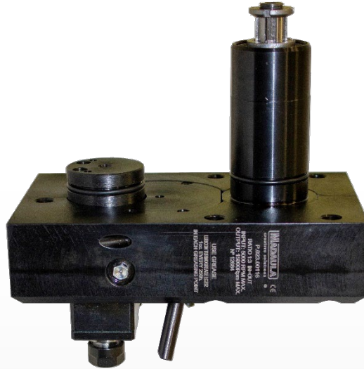
Axial Offset 2 Outputs for DMG Cyl. Ø40 + Gear / ER-11 Ratio 1:3 – IN=OUT / 15.000 rpm Max.
