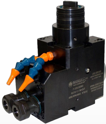
Radial 2 Outputs for FAMAR Cyl. Ø52.8 / ER-20 Ratio 1:1 – IN=OUT / 4.000 rpm Max.
