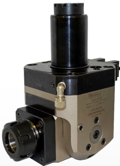
Radial Adjust. 0-90° for BARUFFALDI VDI-50 / ER-32 Ratio 1:1 – IN≠OUT / 4.000 rpm Max.
