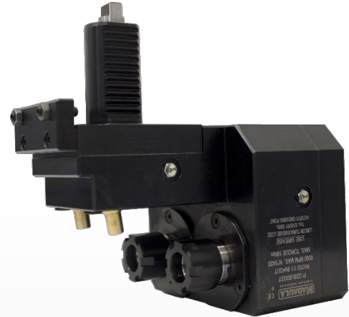
Radial 2 Outputs for HANWHA VDI-40 DIN-1809 / ER-20M Ratio 1:1 – IN≠OUT / 6.000 rpm Max.
