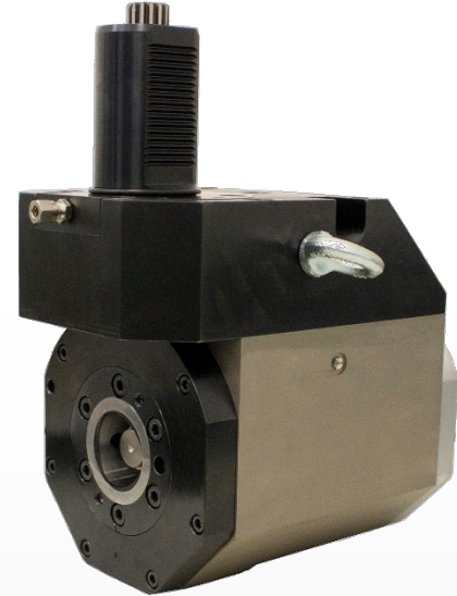
Radial Set-Back IC for GURUTZPE VDI-60 DIN-5482 / CAPTO C6 Ratio 1:1 – IN=OUT / 2.000 rpm Max.
