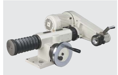
C End face grinding attachment (only 150NC)
