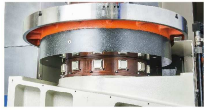
B 德國製靜壓轉盤 Hydrostatic rotary table (Made in Germany)
