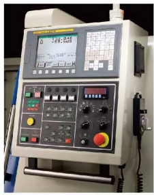
A 發那科控制系統Fanuc Oi-TF controller
