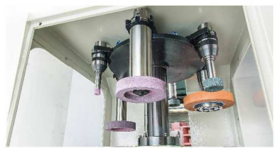
J 刀庫系統(不含砂輪和接桿) Tool magazine(not included wheel & arbor)
