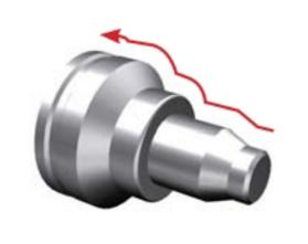
Workpiece Part for mission Cutting vc (m/min) = 160, fn (mm/rev) = 0.13condition ap (mm) = 1.0, wet Insert : DNMG150608-LP (NC3225) Designation Holder: DDJNL2525-M15 ■ Test result Cutting pass/Corner 110 80 NC3225 Competitor
