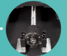
High Precision Ball Screw : X, Y, and Z axes are equipped with precision ball screws, which are pre-load to ensure the best accuracy and minimize the positioning error.
