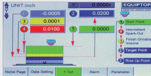
Grinding feed (for rough, fine, and spark-out setting). Min. display unit for Y/Z axis is 0.001mm.
