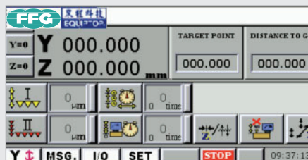
Downfeed ( Rough grinding, Finish grinding, Sparkout setting ) Minimum Display Unit: Y axis 0.001mm / Z axis 0.001mm
