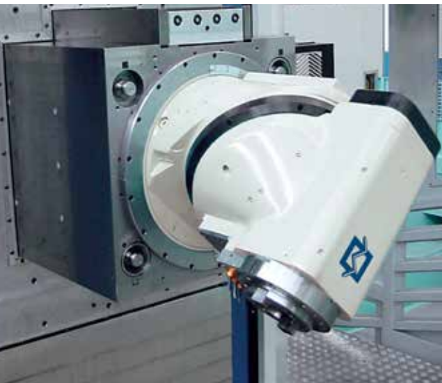
Universal high-stiffness milling head (power 46 kW)
