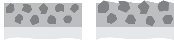
Figure 5: Aim of the sharpening - Creation of grain overhang (micro geometry)
