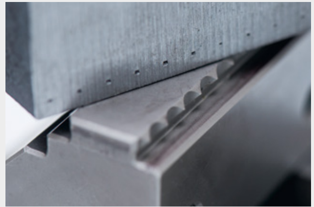
Holding teeth of a conventional vice + indentation in workpiece
